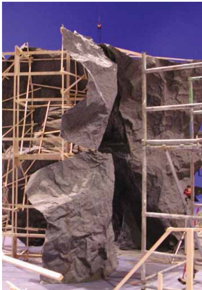
Brusan moulds easily round a light framework to form rocks or cliffs.
