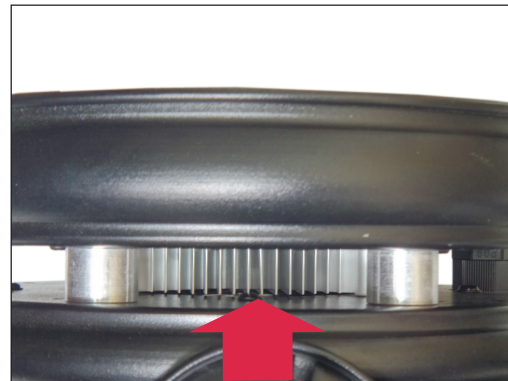
heat sink for better ventilation
